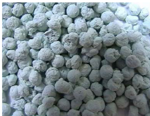
Fig. 7. Exhausted LoFloSorb after 48 hours in a sealed vessel
